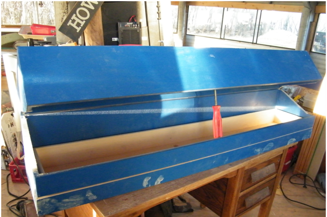
Pre assembled sections all test fitted together– ready for final finish 220 grit sanding and finish coating of paint products to be applied.
